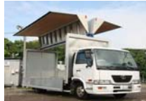
Trailer Truck with "wing" 10,000kg- 13,000kg loading
